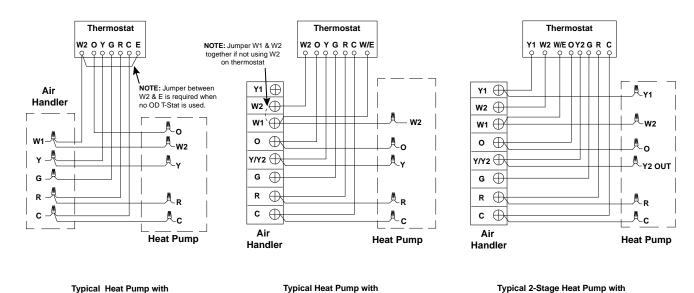
Figure 9. Typical Thermostat Connections
