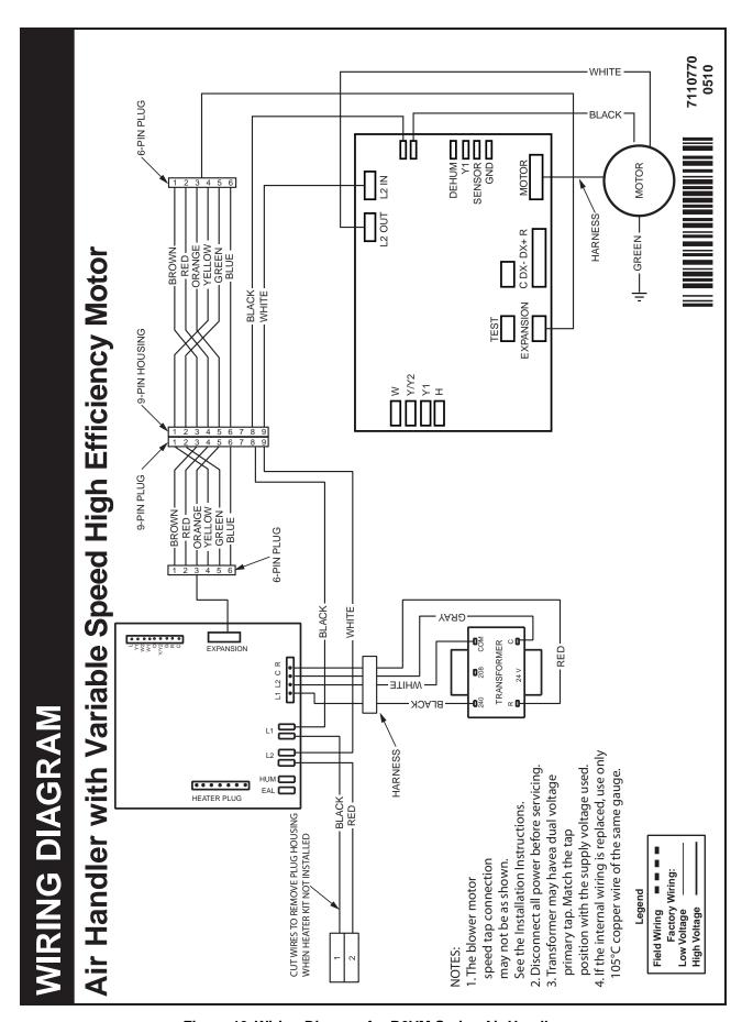
Figure 19. Wiring Diagram for B6VM Series Air Handler
