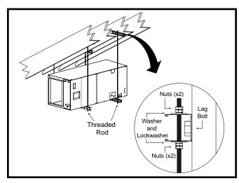
Figure 4. Unit Horizontally Suspended
