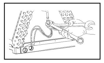
Figure 5. Loosening of Nut & Distributor Body
