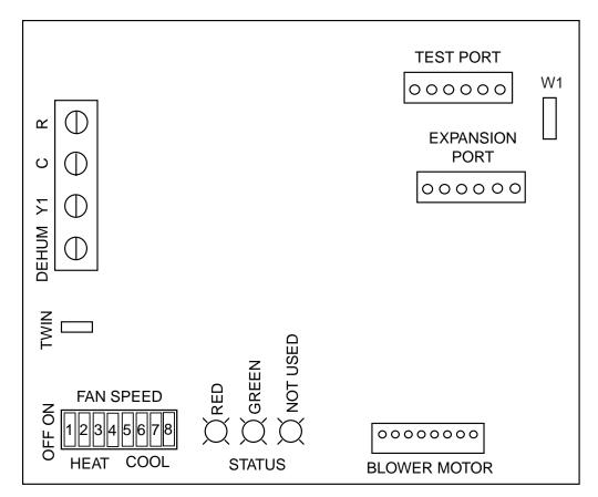
Figure 15. Fixed Speed Motor Control Board
