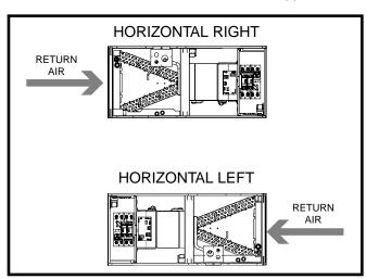
Figure 3. Horizontal Configurations
