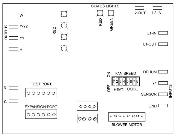
Figure 16. Variable Speed Motor Control Board
