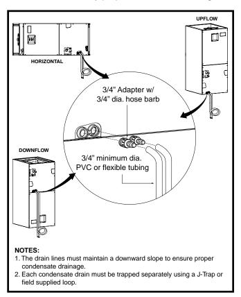
Figure 8. Condensate Drainage Example
