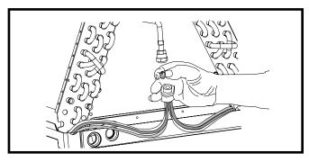
Figure 7. Restrictor Insertion into Distributor Body
