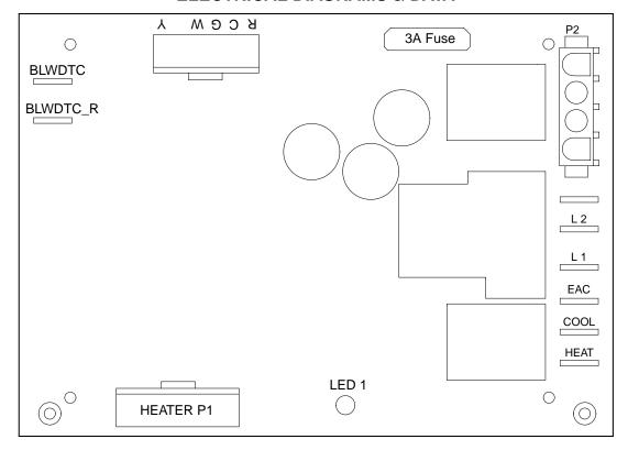
Figure 13. Single Stage Control Board
